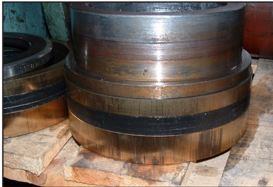
Damaged piston seals and piston head
